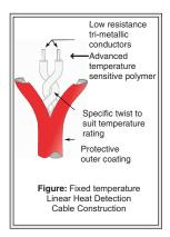
System Sensor Fixed Temperature Linear Heat Detection Cable range consists of a twisted pair of extremely low resistance (.05 Ohm/ft. of twisted pair) tri-metallic conductors, sheathed in new advanced thermal polymers. These polymers are chemically engineered to breakdown at specific fixed temperatures allowing the twisted conductors to make contact and initiate an alarm at the control panel without any calibration for changes in ambient temperatures.
